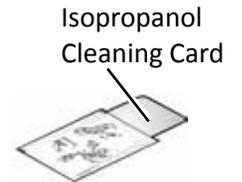
5. Load the cleaning card in the input hopper. Clean the printer immediately. The cleaning card dries out if it is out of its package for more than a few minutes.
