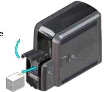
4. Open the cleaning card package and remove the isopropanol cleaning card.
